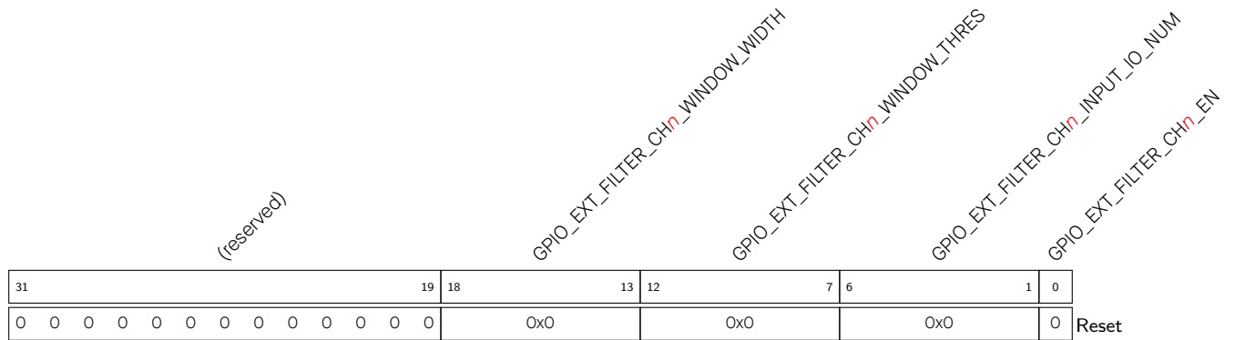
Register 8.47. GPIO_EXT_GLITCH_FILTER_CH n _REG ( n : 0 - 7) (0x0030+0x4* n )
