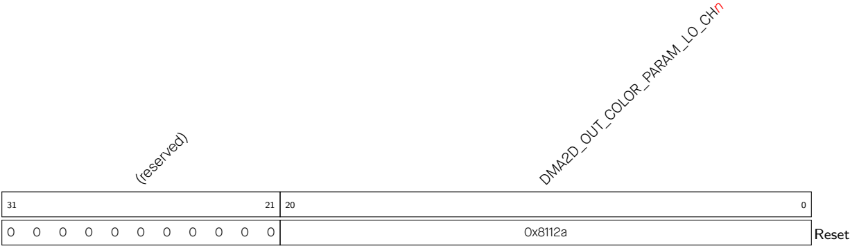
Register 5.13. DMA2D_OUT_COLOR_PARAM4_CH n _REG ( n : 0-2) (0x0060+0x100* n )
