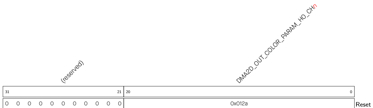
Register 5.9. DMA2D_OUT_COLOR_PARAM0_CH n _REG ( n : 0-2) (0x0050+0x100* n )
