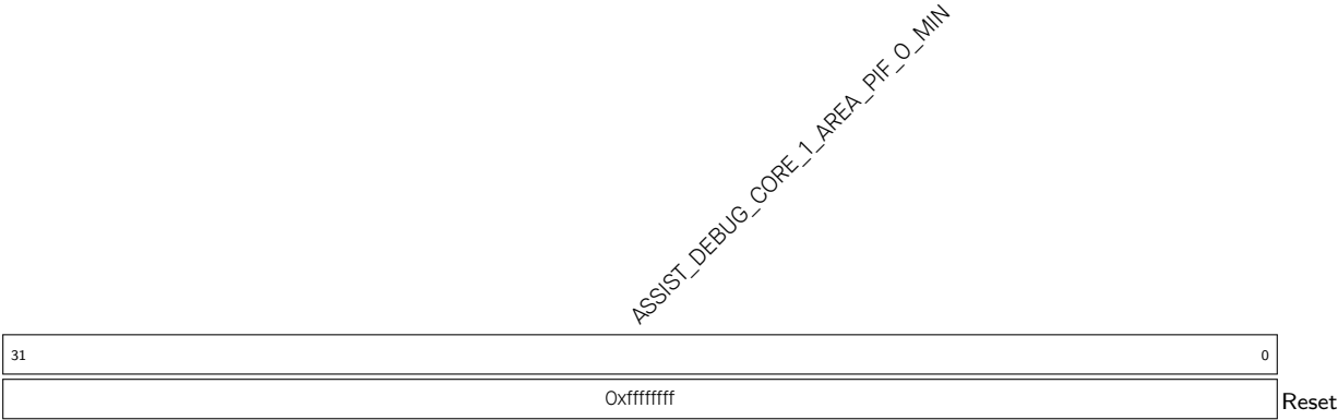
Register 19.53. ASSIST_DEBUG_CORE_1_AREA_PIF_O_MIN_REG (0x00A0)
